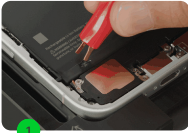
Connect the adhesive tabs to the 9V battery.
